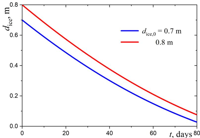
Figure 6. Time variation of ice layer thickness during the ice melting.
