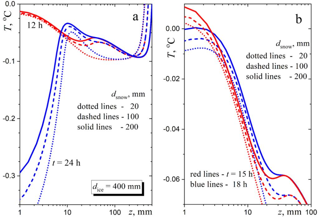
Figure 5. Temperature profiles in the snow and ice layers underneath at different times of the day: a – at noon and midnight, b – in the afternoon.
