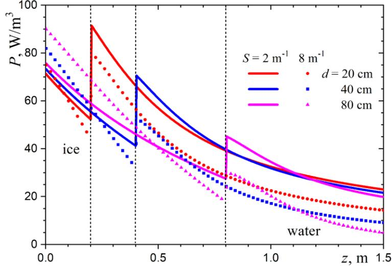
Figure 1. Absorbed radiation power profiles in ice and water at different values of scattering parameter and ice thickness.
