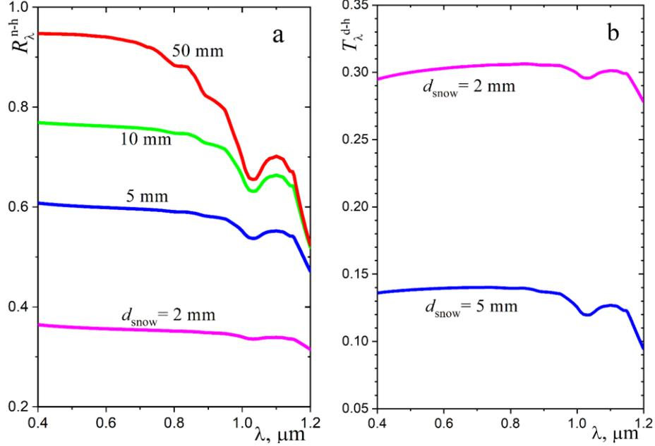
Figure 4. Effect of snow layer thickness on (a) normal albedo and (b) transmittance of snow.
